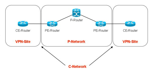
During transport two labels are used: one to identify the 'egress PE', the other one to identify the customer/a particular VPN.
