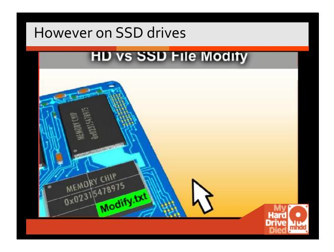
You cannot make a change (cannot edit a file in place in an SSD) within those cells without erasing the state of those cells. Legacy: PBA (Physical Block Address) conversion to LBA (Logical Block Addresses). At lower level, there is a translation table, which converts Physical Block Address to the LBA Block Address, which then supplies the data from the new location.
