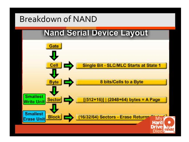
This is a basic chart of memory sizes of existing NAND. If a single bit fails in this block, the entire block is put in a bad block list (128K).
