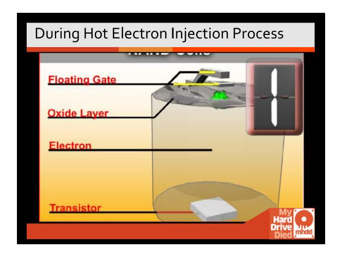
Currently the floating gate is pushing the electron through the oxide layer (hot electron injection), and that will take the state from 1 to 0.
