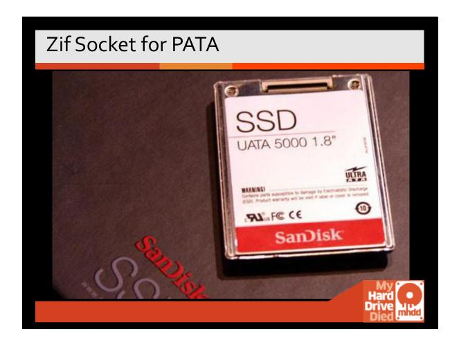
This is a special ZIF socket, which is still a PATA format used by many solid-state disks. The ZIF sockets are very touchy and do not last very long. They are very difficult to connect and generally will only last about 20 connections before failing.
