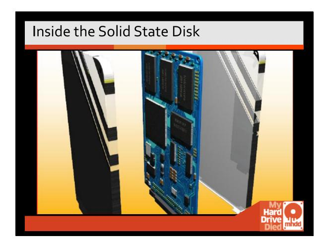
SSD has no moving parts. With no moving parts, solid-state drives are less fragile than hard disks and are also silent (unless a cooling fan is used); as there are no mechanical delays, they usually employ low access time and latency.
