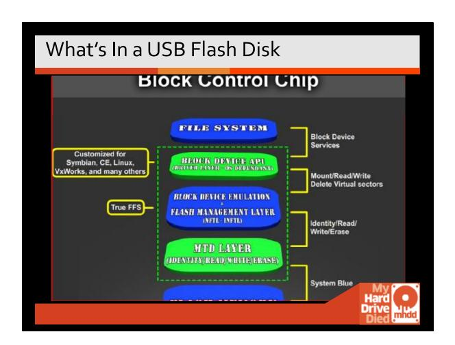
SanDisk bought M-Systems. This is a view of the basic functional implementation of a product by SANDISK to protect the contents of flash memory and is called True FFS.
