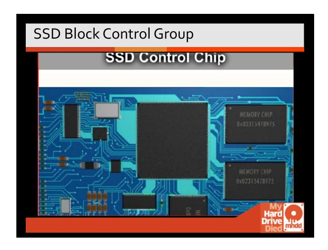
The control chips for SSD drives are much different that USB and have the ability to process data on their own.
