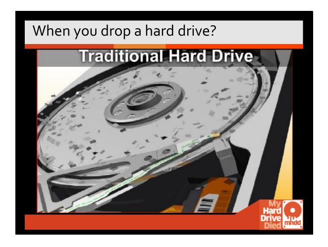
The damage done to a hard drive by dropping it or any kind of fall, is still very destructive for a traditional hard drive.
