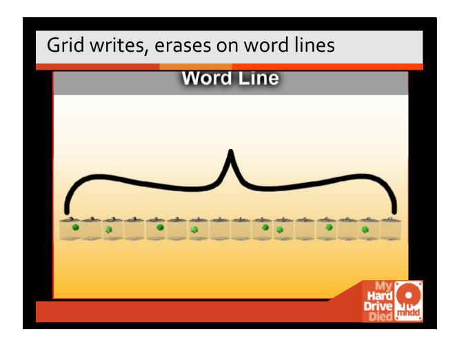
Due to the arrangement in a grid, you can't write to just one line. It must be a group of gates, according to the manufacture.
