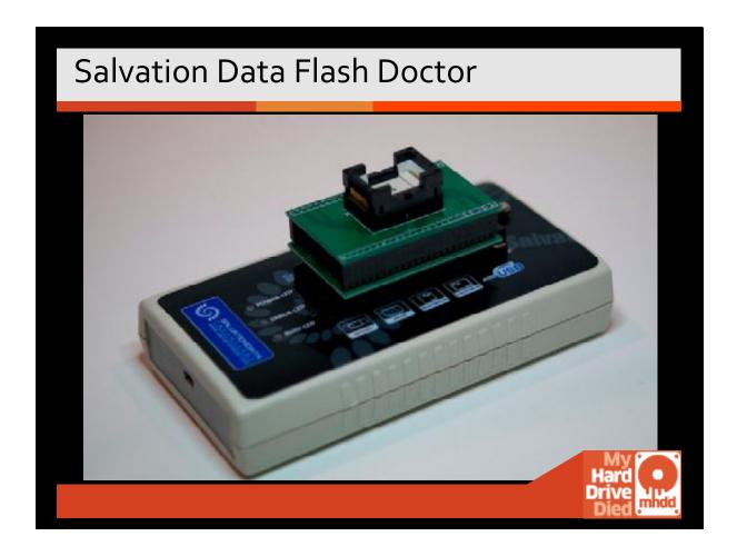
This is Salvation Data's Flash Doctor. This is used for Solid State Repair. You remove the chips, and then image them, and use software to reinterpret what the content was on the device.
