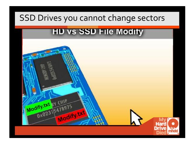
Now the modified file exists at a new location as it cannot be changed in its current location. Then the sector has to be added to the garbage collection routine due to the fact that it cannot be changed or erased in its location. It must be done on the new location.
