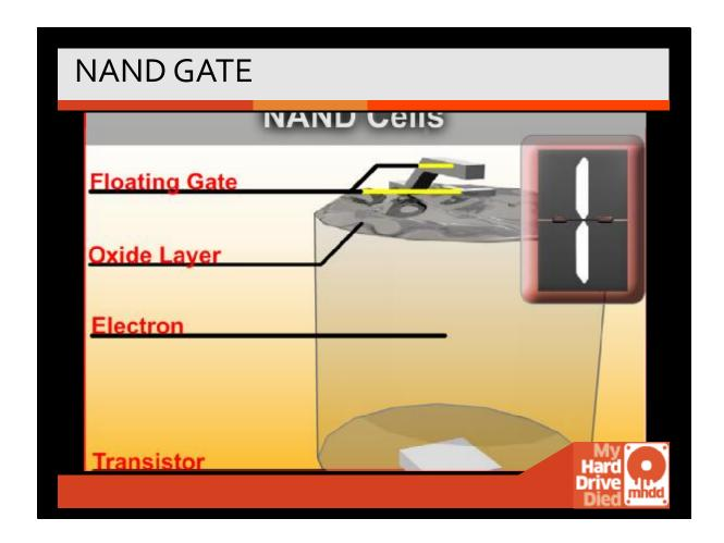
The floating gate itself will push the electron though the oxide layer using a process called "hot electron injection." It will store the electron in the cell. When no content is in the cell and it is empty, its state is One. Usually we would think of that as state zero, but in NAND it is in state One.
