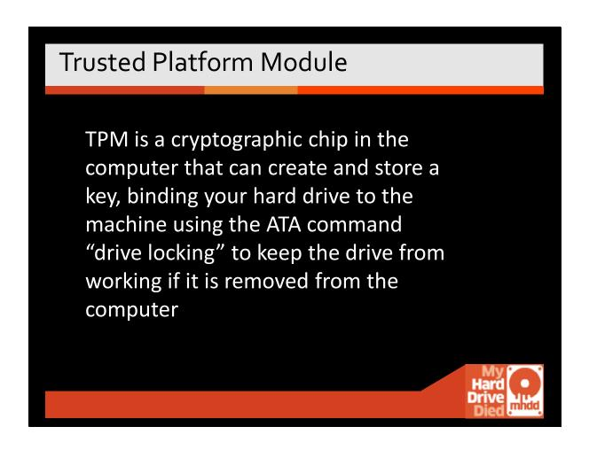
Encryption exists on some SSD and USB Thumb Drives. TPM is a cryptographic chip in the computer that can create and store a key, binding your hard drive to the machine using the ATA command "drive locking" to keep the drive from working if it is removed from the computer.
