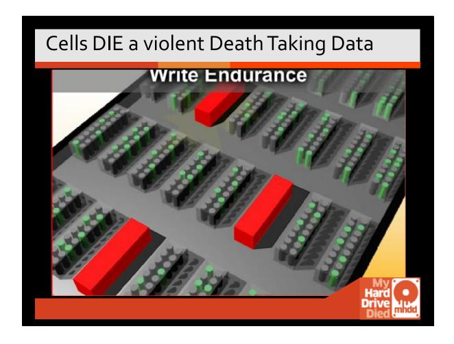
Cells will die causing blocks to be marked bad. In flash-based solid state disks the write endurance is the number of write cycles to a block of flash memory. Once you have met the write endurance limit, the disk may become unreliable or unable to use any of the cells.
