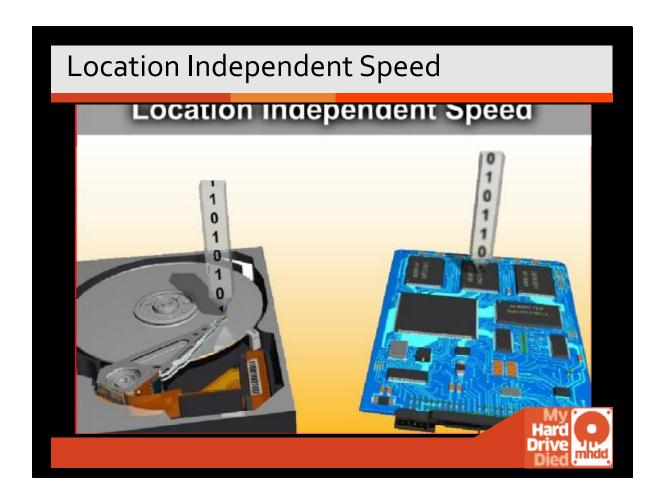
On the hard drive: You have wave forms as disks are being encoded. On solid state disks: Data is stored as 0's and 1's (a lot fewer errors). Hard drives use Constant angular velocity.
