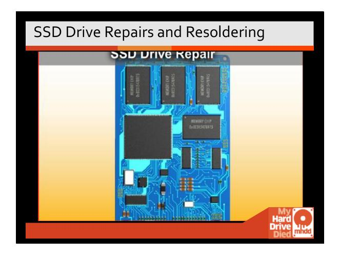
SSD drives are a lot more complex and costly to disassemble and reassemble. The hard part is that you have to carefully de-solder and re-solder all the chips. The expensive part is that you have to destroy another drive just like it to get the board or parts.
