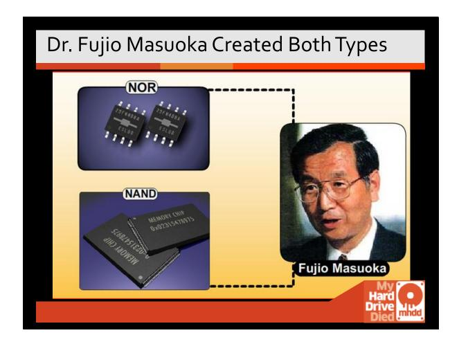
NOR and NAND are the other two types we use most for all SSDs. Dr. Fujio Masuoka was a former employee of Toshiba and is the inventor of flash memory. He also developed the SAMOS memory (stacked gate avalanche injection type MOS) structure. The SAMOS is employed as a memory IC. (<u>http://en.wikipedia.org/wiki/Fujio\_Masuoka</u>).
