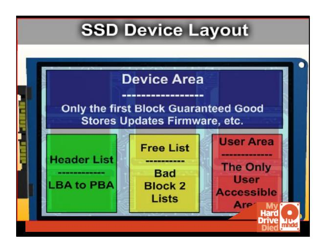
In solid state devices the blocks virtualize all the content over the device itself. The fundamentals of the basic generic table for most devices seem to be in this layout:
