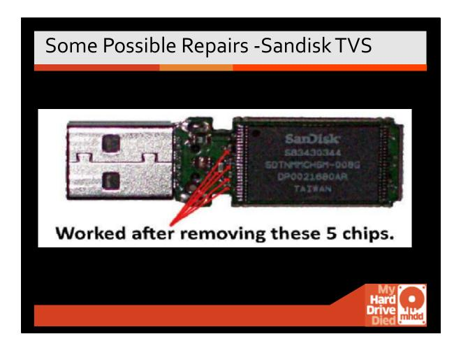
On a hard drive there are chips called TVS Chips (transient voltage sensors) and when they trip the drive stops working to protect itself from power overloads. Same is true of Solid State Drives and USB Thumb Drives. The above is an example.
