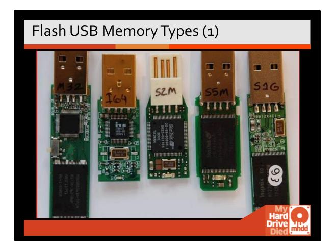
Samples of Flash USB Sticks we have damaged, repaired, and imaged.
