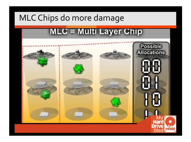
NOTE: They are not separate CELLS just cells CHARGED AT MORE LEVELS – That is why they are damaged more in MLC and TBC (triple bit cells) because they are charged more. They are also as much as 40% slower.
