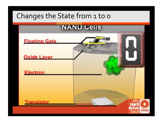
You will notice that the state has not changed to 0. The transistor now will be able to pick up the stored electron and see that there is a charge.
