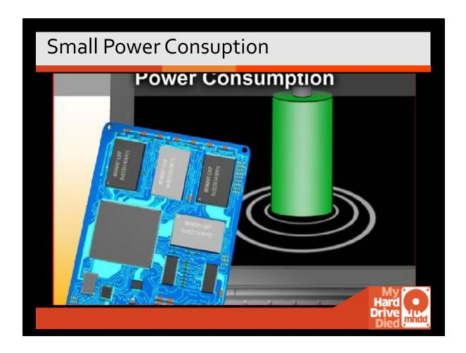
There is a huge voltage differential. An SSD is also faster because there is no spin-up time and it goes straight from one state to another. It's either on or off, inactive or active.
