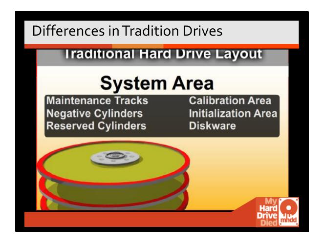
This is a comparison for what is changing on Flash that are legacy items, which seem to no longer be needed on hard drives. Maintenance Tracks is the oldest name. Negative Cylinders is the primary word used; it will read backwards.
