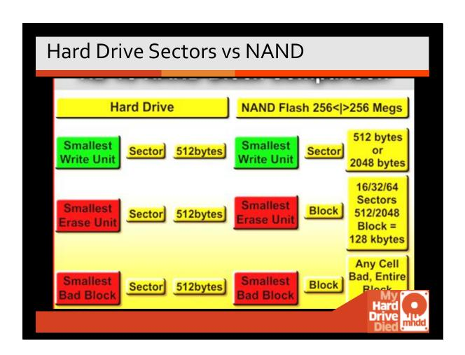
This is a comparison to hard drives and the data sizes, including the smallest bad block. Losing 128k every time one cell dies can cause the disk to shrink over time.
