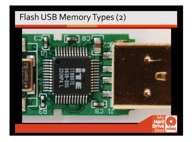
This is an example of the control chip for the USB device.
