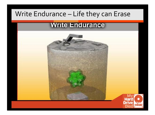
In flash-based solid state disks the write endurance is the number if write cycles to a block of flash memory. Once you have met the write endurance limit, the disk may become unreliable or unable to use any of the cells.
