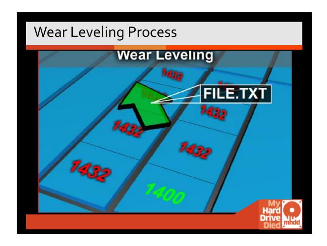
When content is changed it must be moved to a new location before the data can be saved, and then the data will be stacked in the garbage collection queue.
