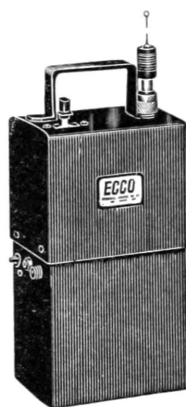
ECCO 10 METER TRANS-RECEIVER Designed for spot frequency use for emergency, CD, and net operation. Completely self-contained including batteries. Transmitter uses 20 meter crystals. Fixed frequency receiver has regenerative circuit. Base loaded 36" antenna. Carbon mike input. 1/2 watt input to final. With 5 tubes. Less mike, headphones, crystal, and batteries. MODEL HT-2. Net $74.50. Z-3 Crystal (specify frequency). Net $3.87. Batteries (2-M30 "B", 1-2F "A"). Net $4.76.
